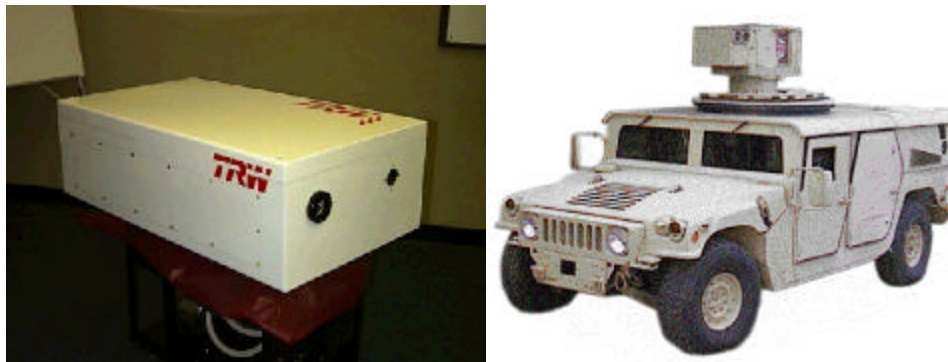
Figure 3. 500-W Laser Delivered to Sparta, Inc. for Ordnance Destruction and the Sparta Zeus System Mounted on a Humvee.
