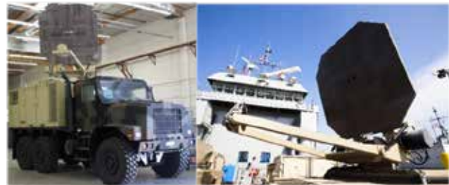
Active denial technology uses mmW emitters to deny, suppress, and move individuals posing a threat in ambiguous situations.
