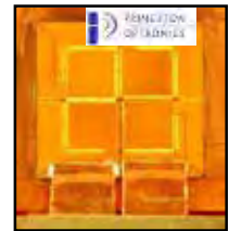
2x2 VCSEL Array 2.7x2.7mm / 530W power
