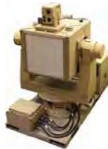
6.8 kW 3300 lb SS-ADT (1W GaN-based MMICs) Skid-Plate Demonstrator with Az/EI Gimbal
