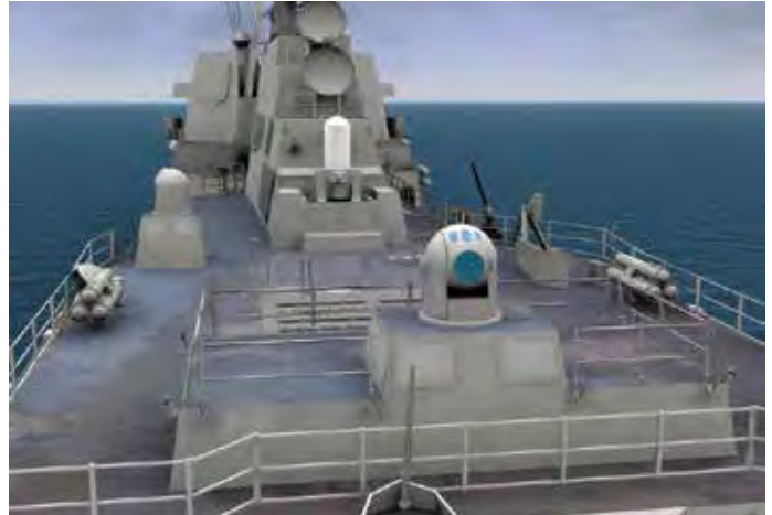
Laser weapon ship integration analyses have been performed to determine potential beam director and subsystem locations for DDG 51.
